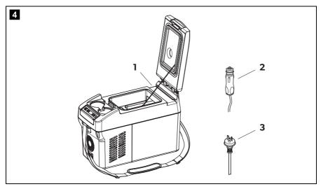
The cooler can be operated with 12 V== or 24 V== or  $100 - 240 \text{ V} \sim$ .
